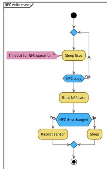
You should always validate your settings by reading the NFC data after the sensor has restarted.
