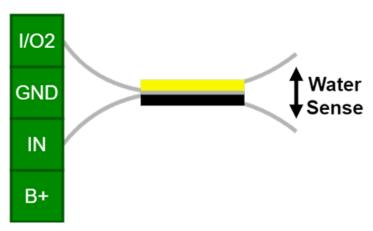
Picture is for illustrative purposes only. The water sense leads does not need to extend the black and yellow wires.
