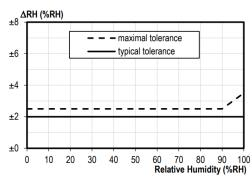
Figure 8. Tolerance of RH at 25°C.
