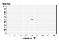
Figure 9. Typical tolerance of RH over T.
